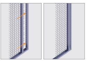
4. Slide the bar and the rule towards the starting rule until the horizontal bars of the bar stop against the edge of the starting rule. Screw the rule to the top and bottom rail.
