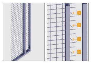
3. Bend every third horizontal bar as much as possible upwards or downwards using manual force and the EGM installation tool.
