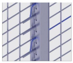
**LOCKING OF BARS, WALL CLASS 2**Every third horizontal bar should always be bent to lock it to the rules in which the bar is placed.
