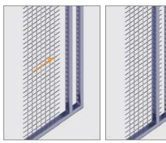
Fold the first bar between the ceiling and floor rail and slide it through the perforated edge of the rule until it stops.
